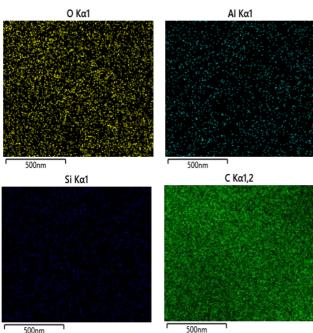
**Gambar 4**. Hasil SEM-EDX Membran PSF-Zeolit 200 ppm
