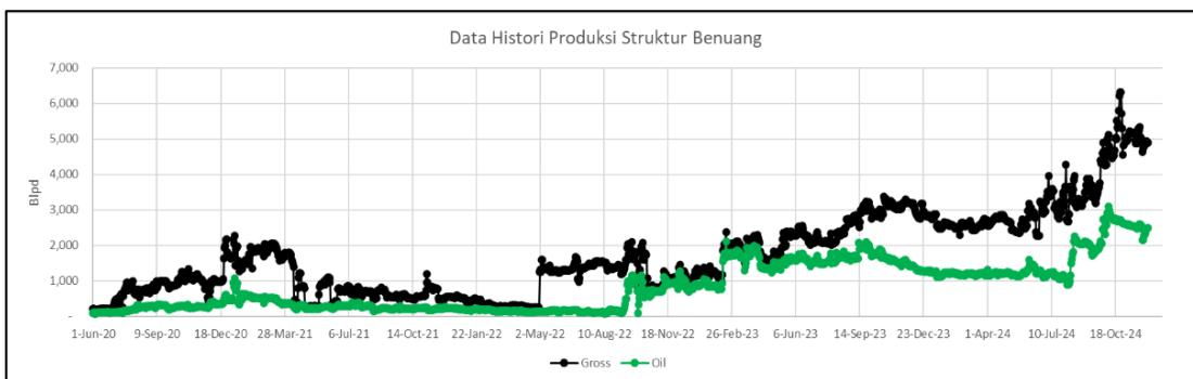
As performance declines due to reservoir pressure depletion, artificial lift methods are required. Well BNG-X3 has shown such decline, having ceased production since April 2023. Despite this, it retains remaining reserves of 60.18 MBO, with economic calculation it is justify to install artificial lift implementation.
