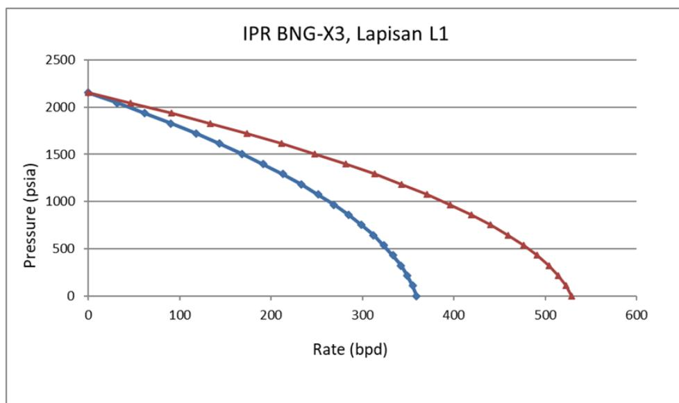
From the data of P Res, Q and Pwf, IPR can be constructed as above (blue line) the red line is the IPR from initial condition, Qmax is estimated at 368 BLPD. A target production of 294 BLPD (80% of Qmax) was set, aiming for 100 BOPD net oil with 66% WC.
