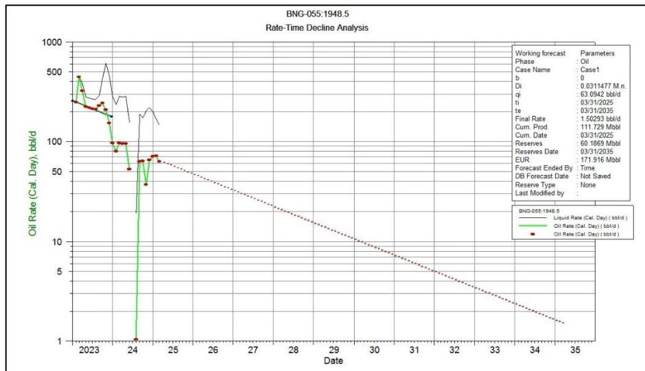
As of now, 111.729 MBO has been produced, leaving 60.18 MBO still potentially be produced.
