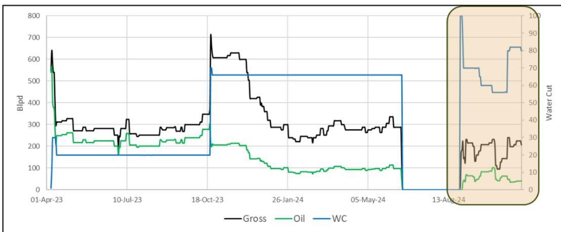
The HPU-installed Well BNG-X3 demonstrated the following production characteristics during the five-month monitoring period. Average gross production: 200 BLPD (barrels liquid per day) and water cut fluctuation: 57% to 87% (showing significant variability). Three engineering perspectives study was held to assess the result:
