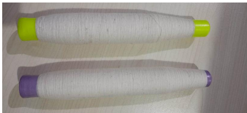
Figure 2. Representative PV 30 yarn samples produced under eccentric and concentric roller conditions.
