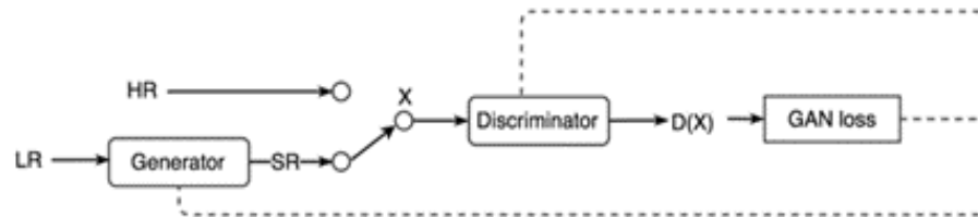
Figure 2. Network design for the generator and discriminator Source: Long, Xinyue et al. [9]
