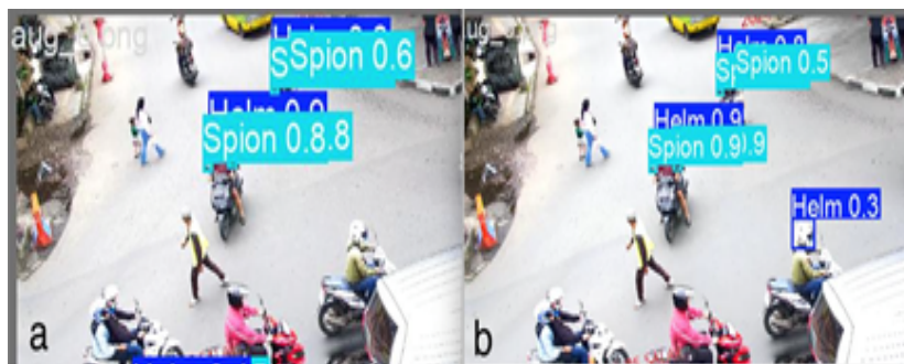
Figure 7. Comparison of Helmet and Mirror Detection Results (a) Without ESRGAN, (b) With ESRGAN
